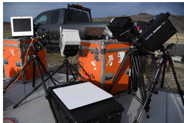
Figure 38: Left to right, the three COTS SWIR meters (SWE, NOR, CAN) and a commercial VNIR PR-745 spectroradiometer.
