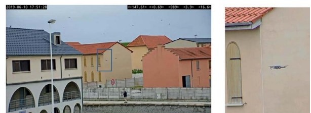
Figure 39: Example of clutter urban environment in the visible band. A DJI Mavic 3 can be seen in the middle of the image, which can be difficult to distinguish from the birds.
