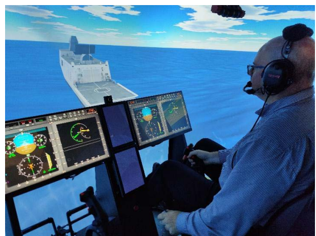
Figure 31: NATO Generic Rotorcraft approaching the NATO Generic Destroyer for a simulated deck landing.
