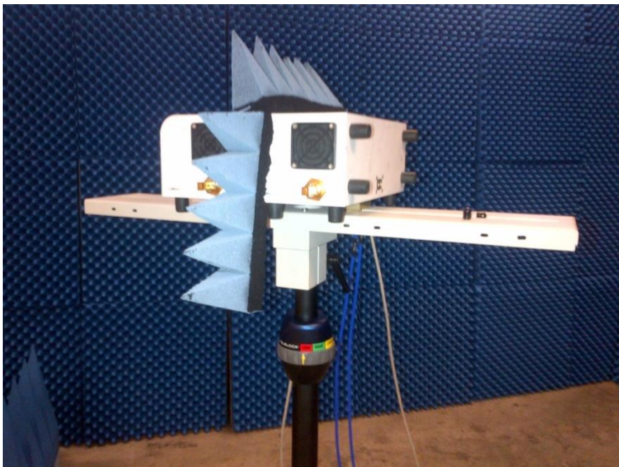
Figure 3: Transmitter/receiver of the Cognitive Radar Engineering Workspace (CREW) at The Ohio State University.
