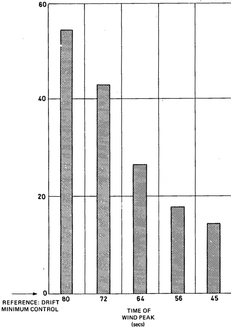
Fig. 5-17 Reduction of maximum bending moment: statistically - designed controller
