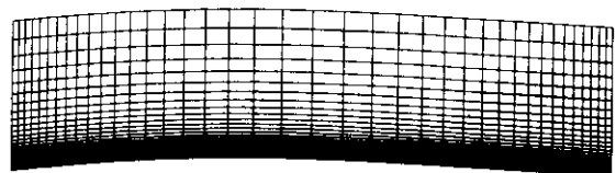
b) GRID NEAR WING SURFACE, Y/S=0.44 (70 CELLS IN NORMAL DIRECTION)
