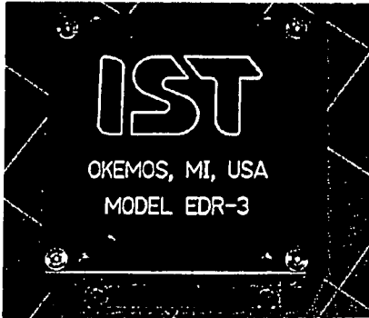
Figure 1 Impact Recorder Chosen for Use In the MSTRP Indy Car Crash Investigation Study.
