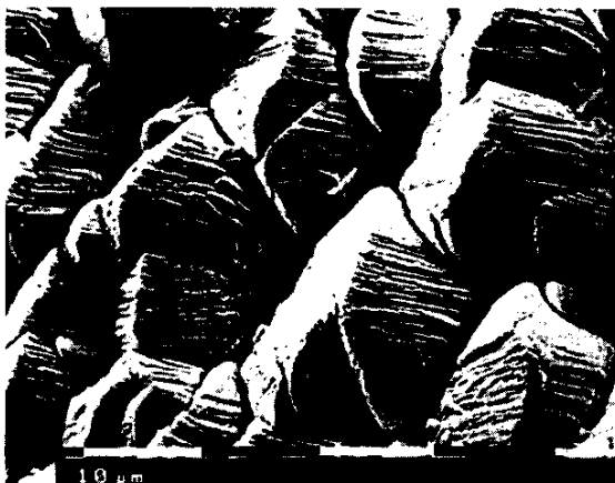
Figure 7: Surface of YPSZ TBCs: a) 980°C; 12rpm; b) 1050°C; 30rpm
