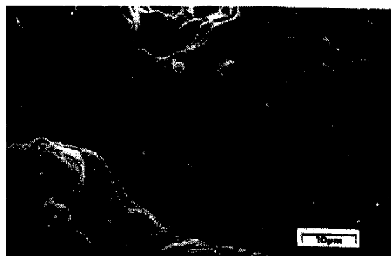
Figure 9 Scanning electron micrograph of the surface of a plasma sprayed TBC showing the high surface roughness and undulating nature of the surface.
