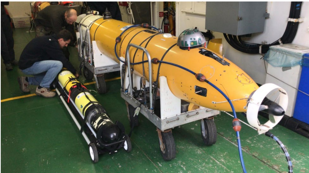
On-deck preparation of an acoustic buoyancy glider (left) and an autonomous underwater vehicle before deployment during DANS19 sea trial
