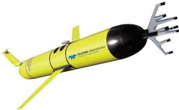
Figure 18: Artist's impression of a Slocum glider equipped with a volumetric array.
