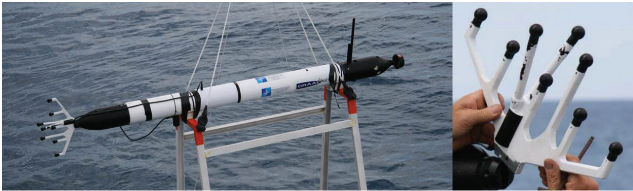
Figure 16: Wave estimation payload, with integrated inertial measurement unit, gyroscope, accelerometers and compass.
