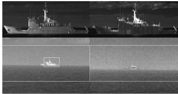
Figure 7: Signature management system: OFF (left), ON (right).
