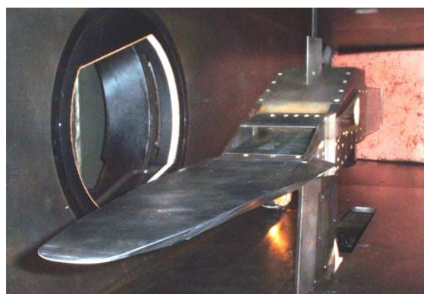
Fig.4 – Mach 2/Mach 8 variable geometry air inletested in ITAM windtunnel
