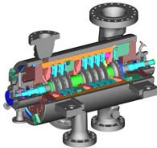
Figure 8: Cut-Away View of a Centrifugal Compressor.
