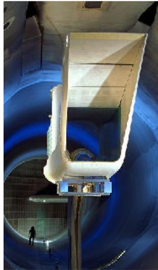
**Figure 1: Boeing / SAMPSON Programme SMA Actuated Intake**
