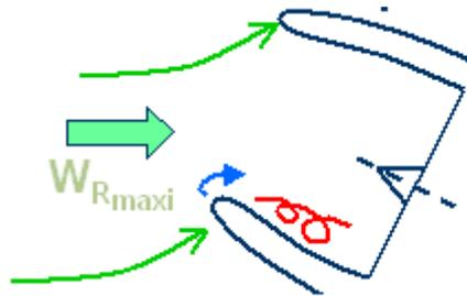
Figure 2: Intake Separation at High Incidence with Thin Intake Lip
