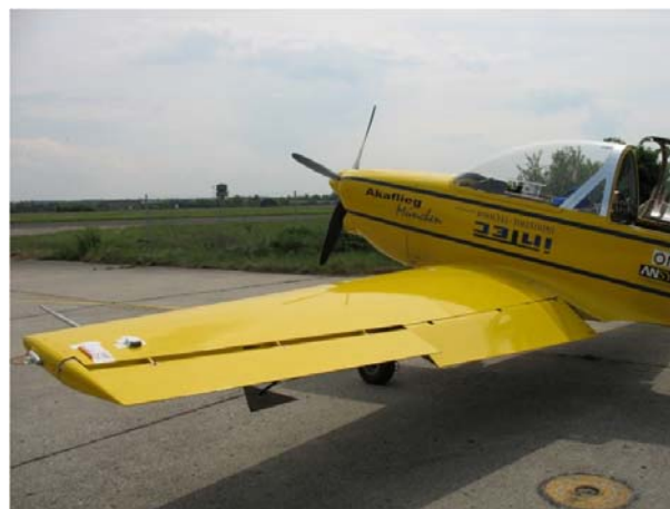
Figure 9: Mü30 flight test: Aircraft Mü30 “Schlacro” with GPS logger mounted on left wing tip
