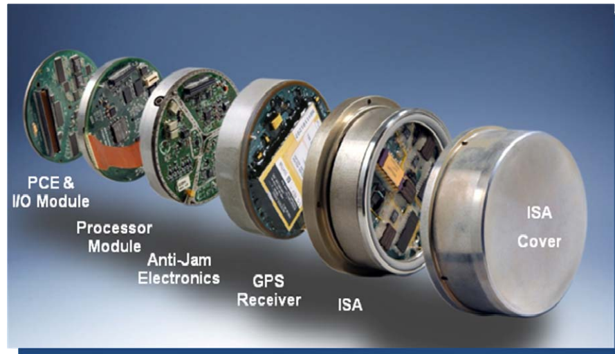
Figure 6: Low Cost Guidance Electronics Unit.
