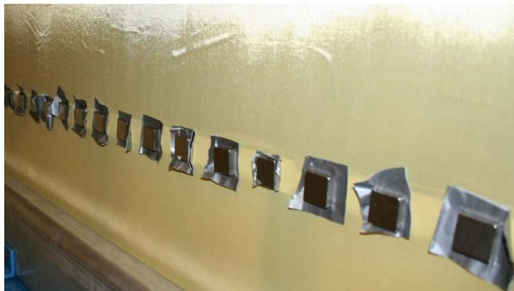
Figure 4.2-5. Rare-earth magnets used to maintain contact between the acoustic windows and the side edges of the test section floor and ceiling, VTSWT.
