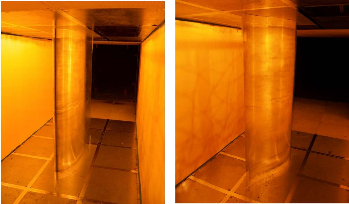
Figure 5.5-1 DU91-W250 airfoil model mounted in the VTSWT hybrid anechoic test section.
