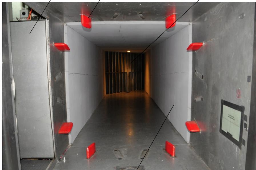
*25-mm thick Melamine foam thickening to 50mm near turning vanes*
