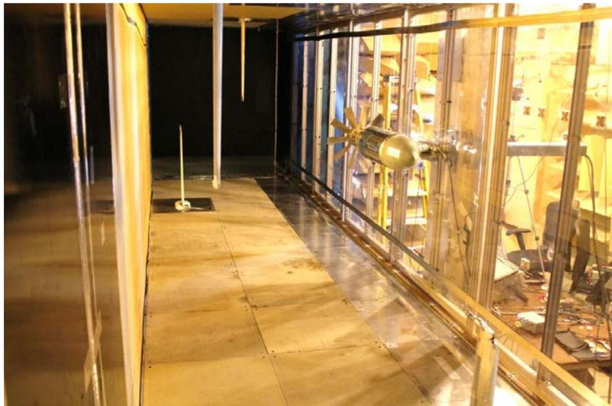
Figure 4.1-2. The VT Stability Tunnel in hemi-anechoic configuration. The transparent wall on the right is used to grow a thick turbulent boundary layer ingested into the rotor system shown. The transparent wall replaces the starboard side acoustic window.
