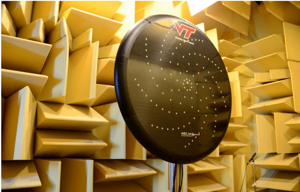
Figure 5.4-1 117-microphone phased array system. Photo courtesy Patricio Ravetta, AVEC Inc.
