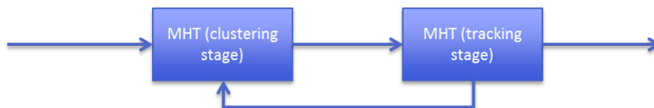
Figure 3-2: A practical two-stage approach to redundant-measurement MHT.
