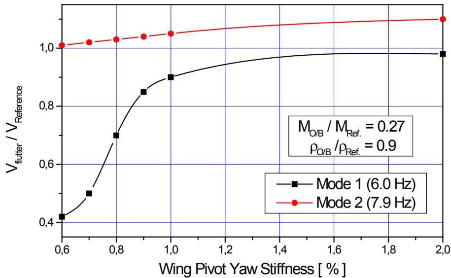
Figure 15: Flutter speed versus wing pivot yaw stiffness.
