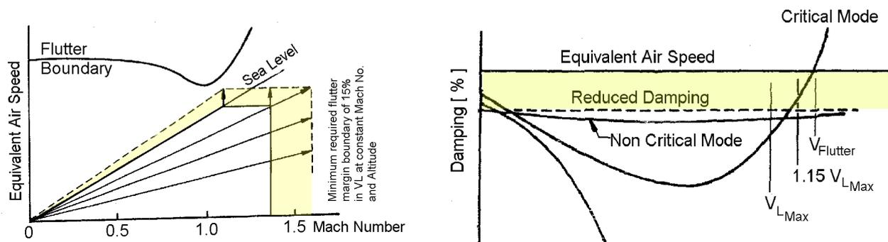
**Figure 3: Graphical Representation of the Flutter Requirement MIL-A-8870.**
