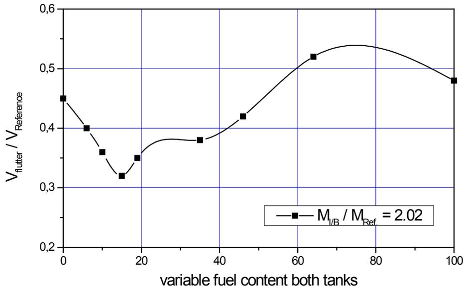
Figure 9: Flutter speed versus symmetrical tank emptying.
