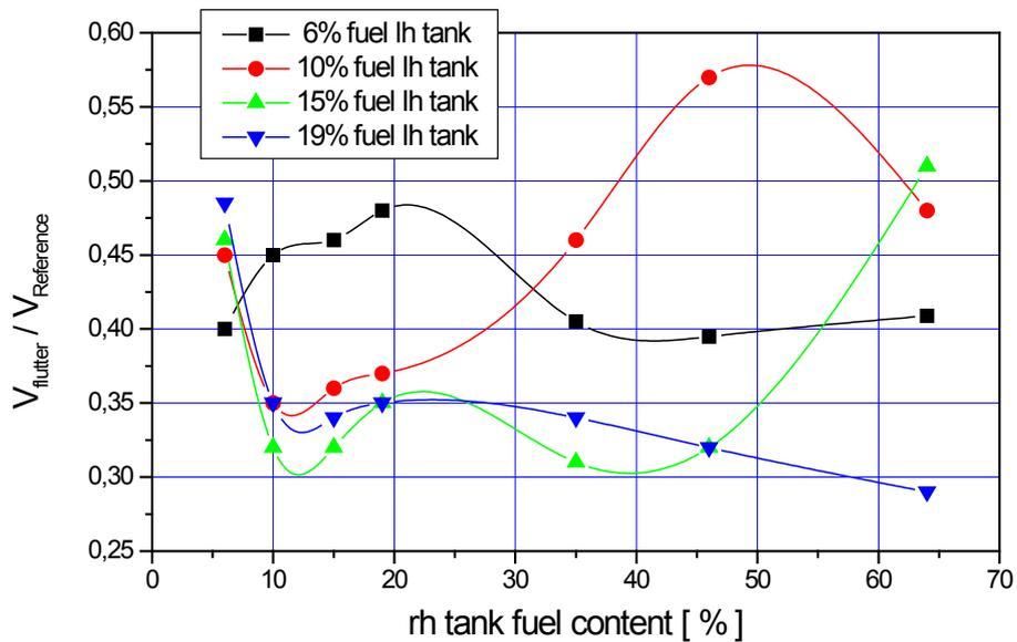
Figure 10: Flutter speed versus asymmetrical tank emptying.
