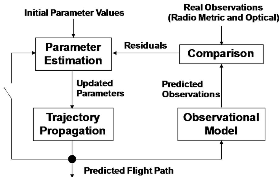
Figure 3: Orbit Determination Process.
