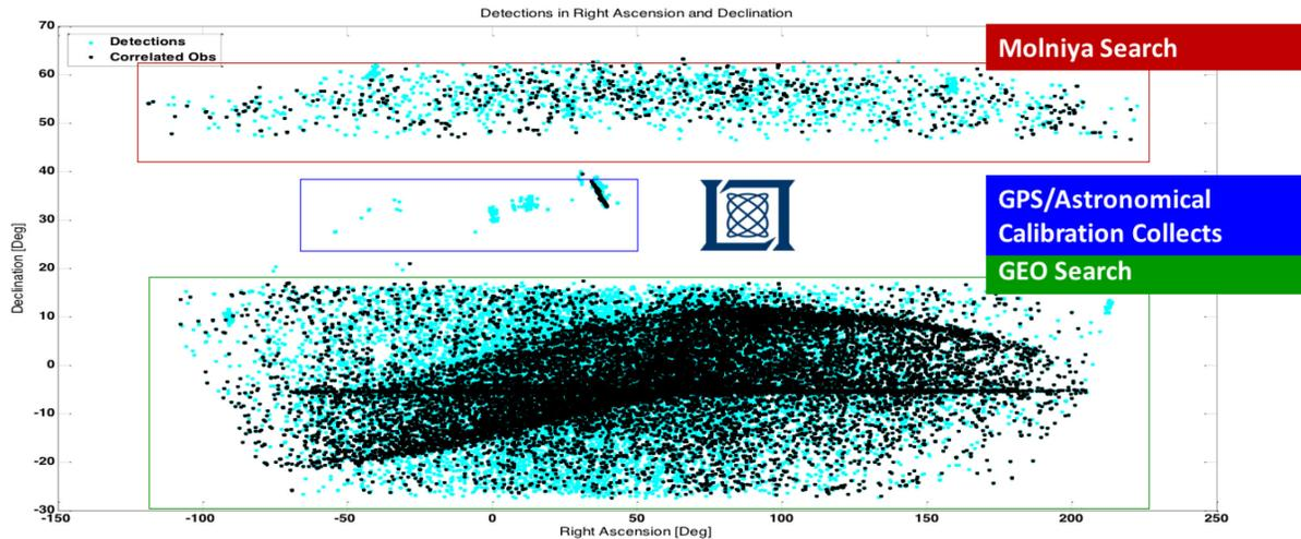
**Figure 5: Correlated vs. Uncorrelated Detections from the Space Surveillance Telescope (SST).**
