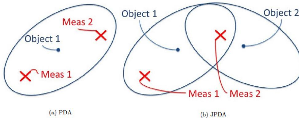
Figure 7: Probabilistic and Joint Probabilistic Data Association.
