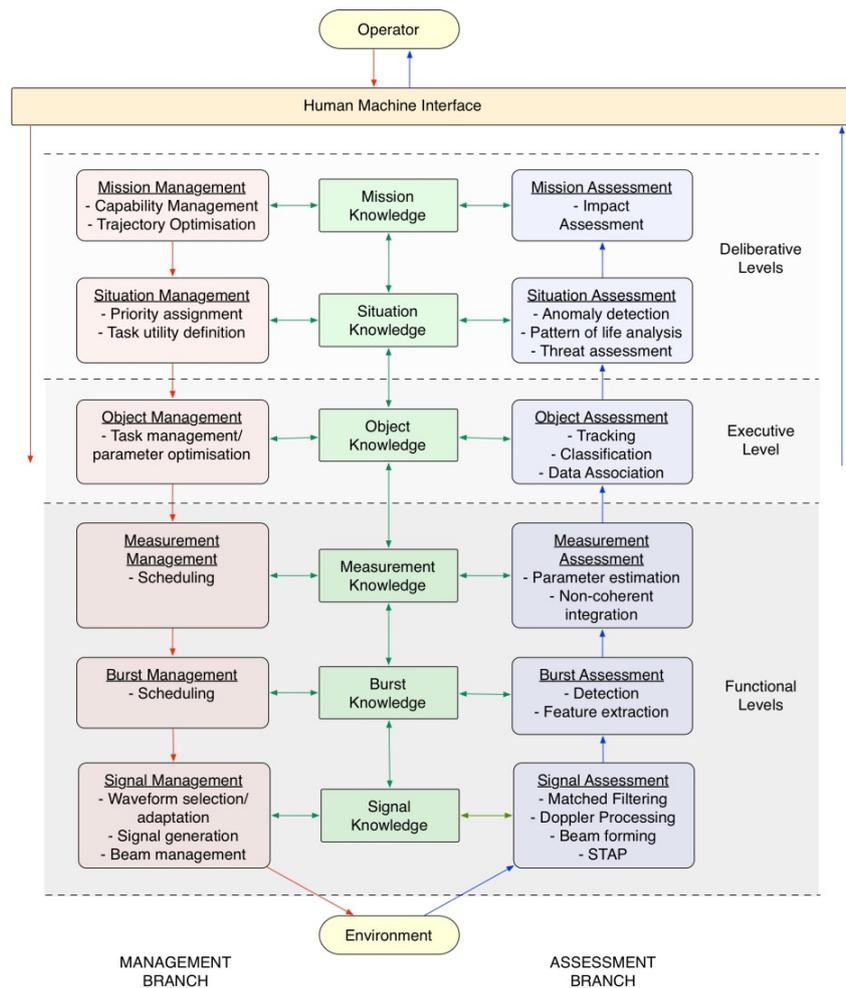
**Figure 1-1: Cognitive Radar System Architecture.**
