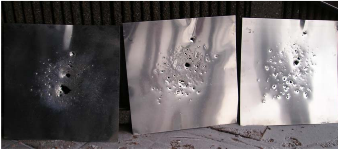
FIGURE 7: Damage of a plate array target due to a PELE penetrator.
