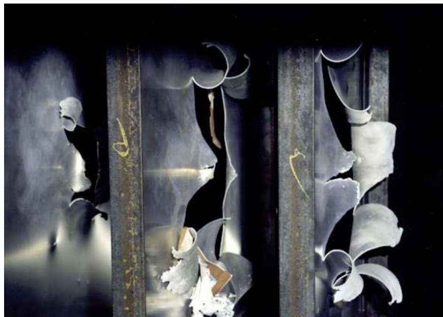
FIGURE 6: Damage inside a target plate array due to a frangible penetrator.
