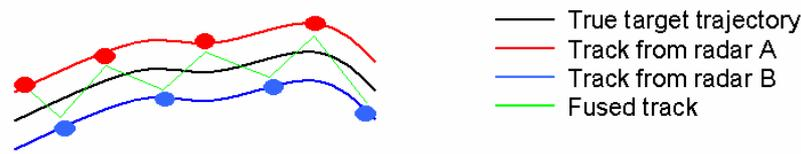
Figure 10: Illustration: Due to Bias, the Fused Track has a Saw Tooth Shape.
