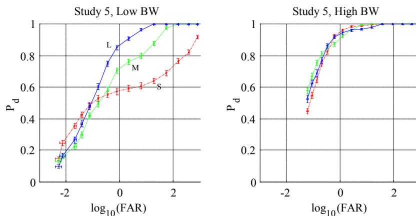
**Figure 9: ROC curves for study one. Left: Low bandwidth (27-50 MHz); Right: High bandwidth (30-80 MHz). Legend: small (dash dot), medium (dash), and large (solid) targets. 23 image pairs were analyzed, including 460 small, 368 medium, and 322 large targets. FAR is in  $\text{km}^{-2}$ .**
