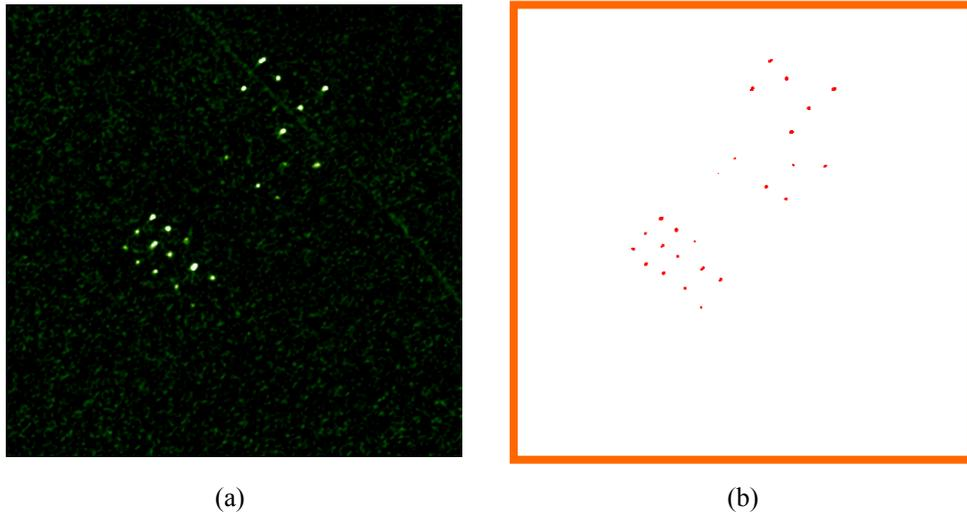
Figure 7: CARABAS-II SAR change detection result from the image pair in Figure 6. (a) Change image based on linear Bayesian classification; (b) After CFAR detection.
