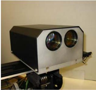
**Laser source:** 1.54  $\mu\text{m}$  - erbium fiber laser
