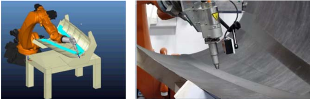
Figure 14: Automatic plasma treatment prior to bonding
