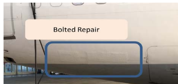
Figure 4: Bolted fuselage repair
