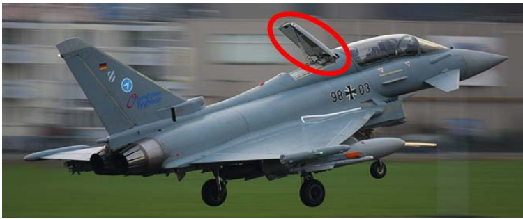
Figure 6: Eurofighter Typhoon (EFA) with deployed airbrake
