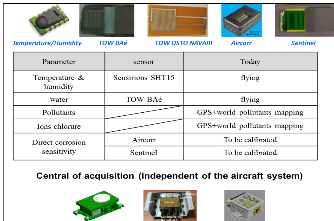
Figure 6 : sensors and equipment for corrosive environment monitoring
