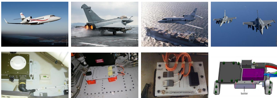
Figure 5 : sensors installation to monitor corrosion severity during new protections experiments
