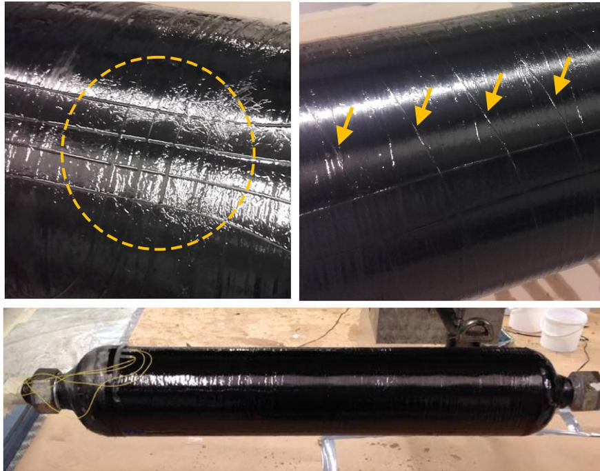
Figure 1: Embedding optical fibres during the manufacturing of carbon fibre COPVs [5].
