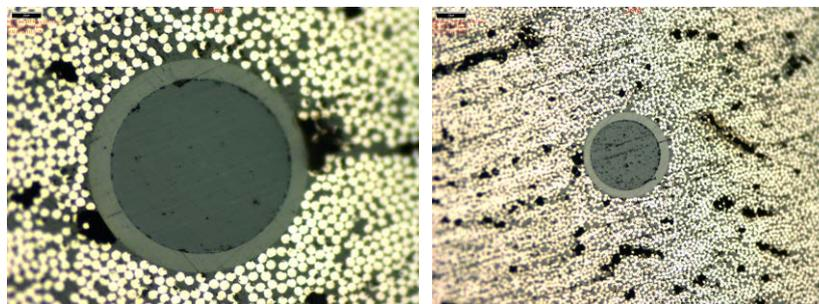
Figure 3: Micrographs of OFs embedded nearly parallel to surrounding carbon fibres.
