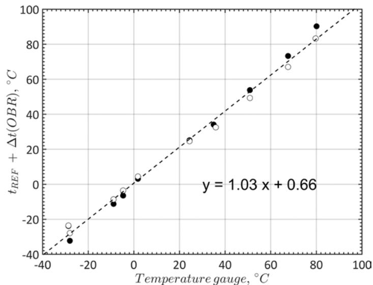
Figure 2: Ambient temperatures measured by the optical fibre sensor and a conventional temperature gauge.
