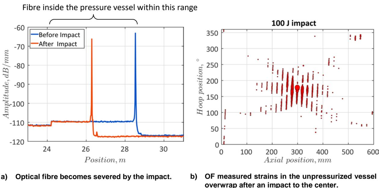
Figure 4: Identifying the impact locations in pressure vessels [5].
