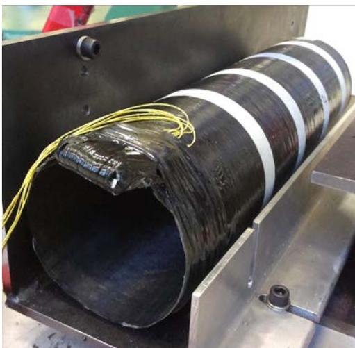
**a) Instrumented composite cylinder.**
