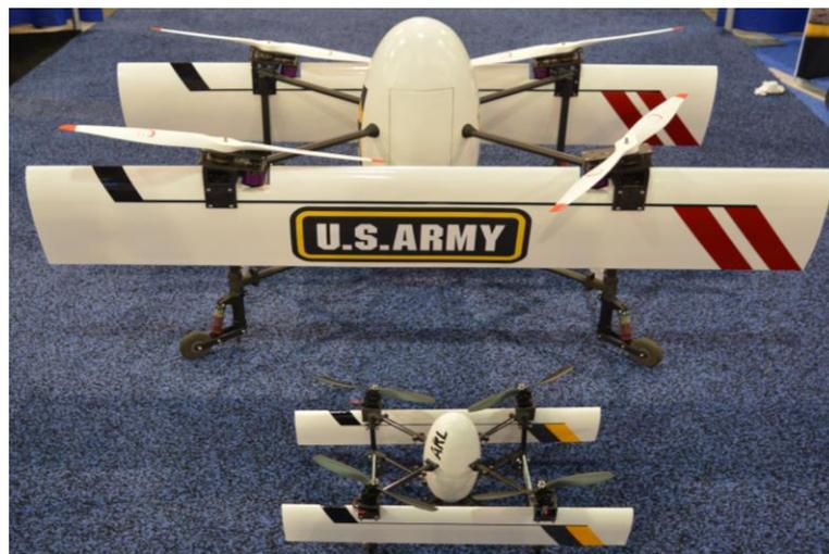
**Figure 1.1-1 Army Research Lab's CRC-20 (top) and CRC-3 (bottom) quad-rotor biplane tailsitter UAVs.**
