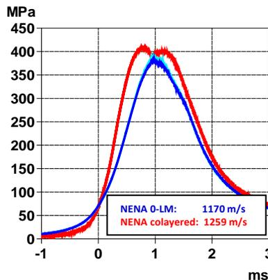
Increase of 15% in muzzle energy with the co-layered propellant at equivalent maximum pressures
