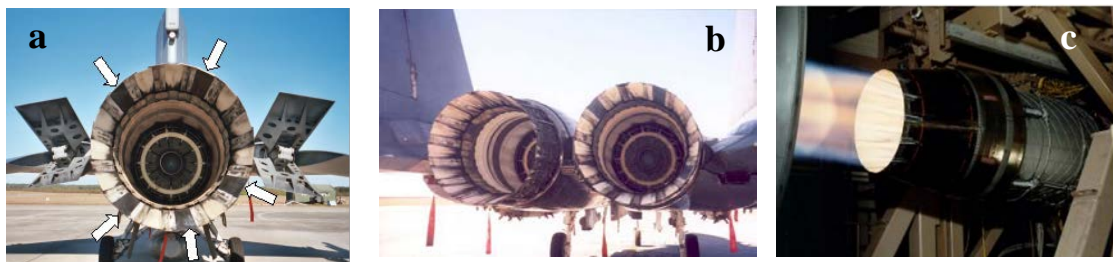
Figure 4: CMCs seals, (a) McEntire JNGB F-16 aft end showing the exhaust nozzle, (b) F-15 at Mountain Home AFB showing the exhaust nozzles of both F100 turbine engines, (c) F100 Ground test
