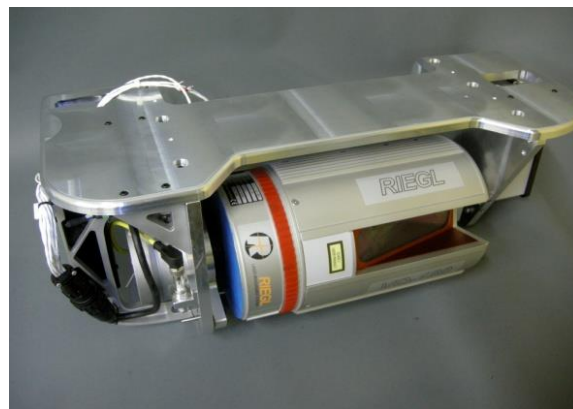
Figure 3: Piasecki Aircraft RIEGL VQ-180 LIDAR
