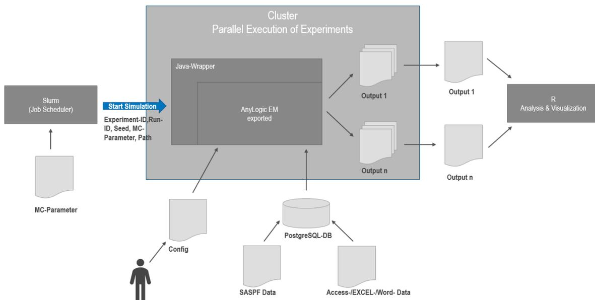
Figure 3-6: Software architecture for the Monte-Carlo experiments on the cluster
