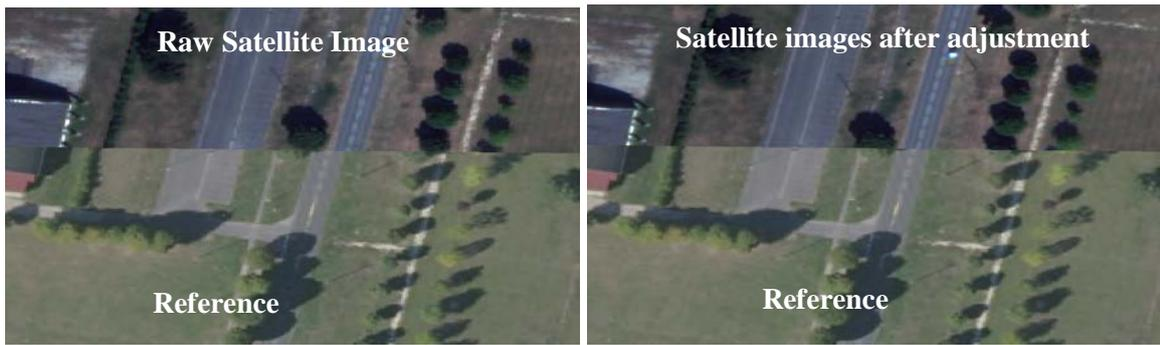
Figure 3: Problem of alignment between a reference and a raw image and automatic alignment.
