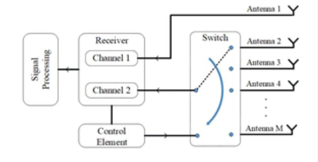
Figure 3 – Array antenna with switched receiver system
