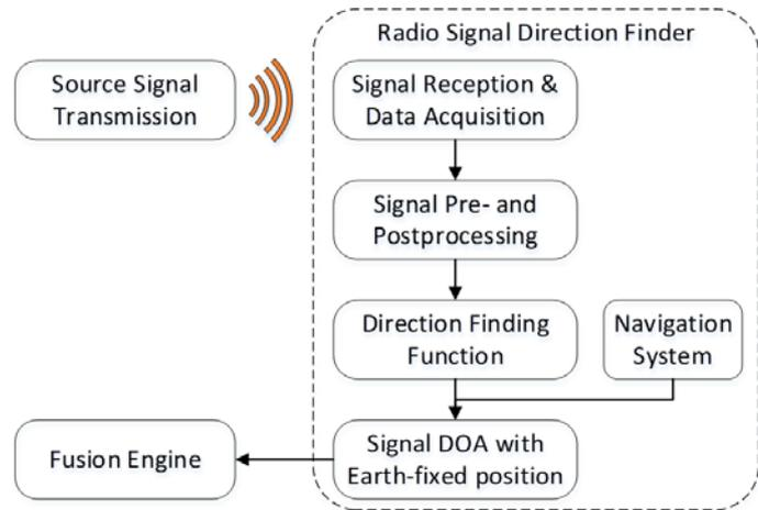
Figure 4 - Functional block diagram of a RF DF
