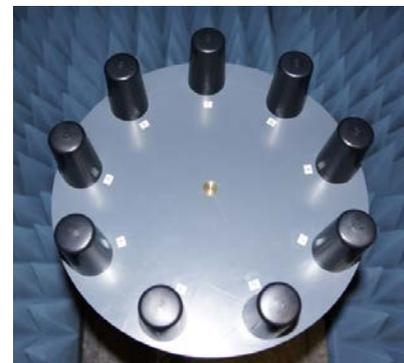
**Figure 2 - Uniform circular antenna array**
