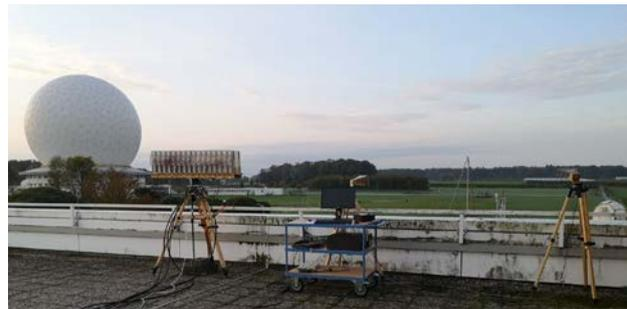
Figure 12 - Passive radar system components set up on the roof of a building
