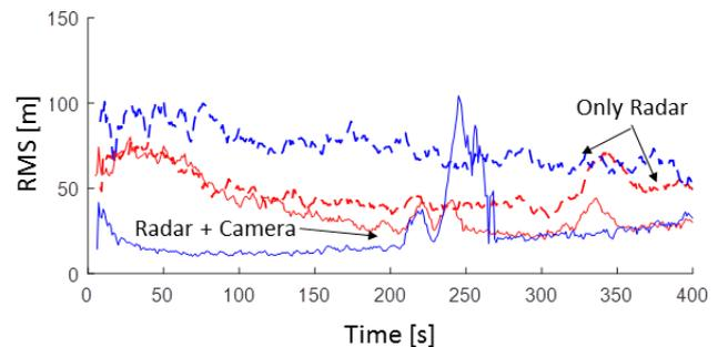
Figure 20 - Root mean square error for each of the targets
