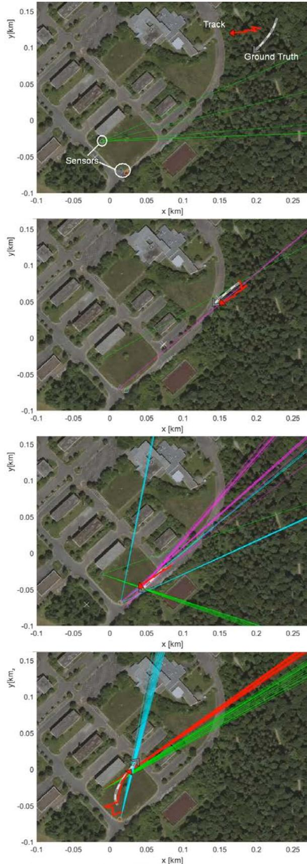
**Figure 221 - Fusion Engine results: Track initialization with radar (a), Track refinement with RF (b), Track refinement with EO/IR sensors (c), Track continuation after flying through the sensor shadow (d)**
