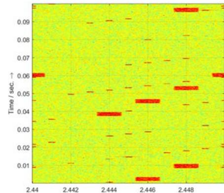
**Figure 1 - Spectrogram of radio signals of UAV application**
