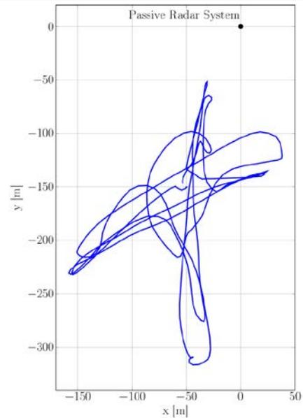
Figure 13 - Cartesian course of UAV flights logged during experimental trial
