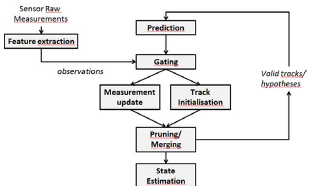
Figure 18 - Multi Hypotheses Tracking block diagram
