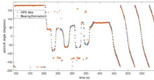
Figure 11 - DoA estimation results (orange dots) for azimuth angles compared with ground truth (blue dots)
