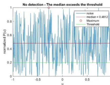
Figure 10 - Noise data and false bearing estimation
