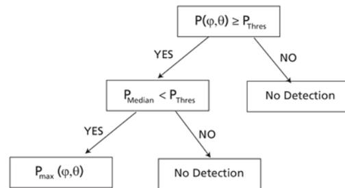
Figure 8 - Flowchart of the second detection method
