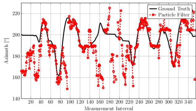
Figure 166 - Azimuth of UAV from ground truth and corresponding state component of TbD particle filter.
