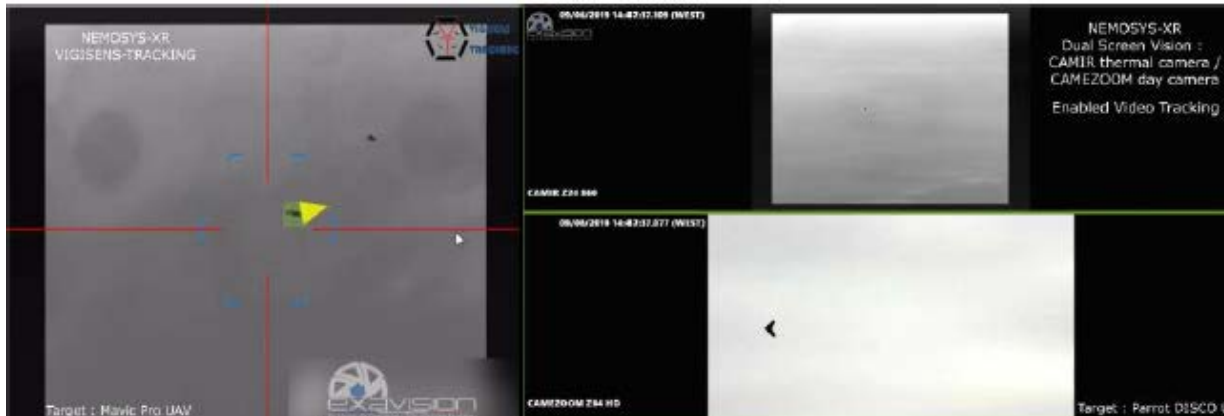
Figure 20 Left IR tracking with NEMOSYS-LR, Right: Illustration of fixed wing detection using EO/IR NEMOSYS camera at 200-300m
