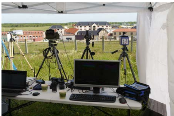
Figure 11 RMA sensor setup at the UAV base, from left to right MATIS (MWIR), FLIR SC640 (LWIR), FLIR SC7600 (MWIR)
