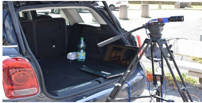
Figure 9 Allied Vision GT1920 mobile camera
