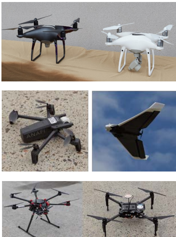
Figure 5 Top: DJI Phantom 4 black and white Middle: Parrot Anafi microdrone and Parrot Disco fixed wing UAV Bottom: Modified DJI S900 hexacopter and DJI Matrice 100 quadcopter
