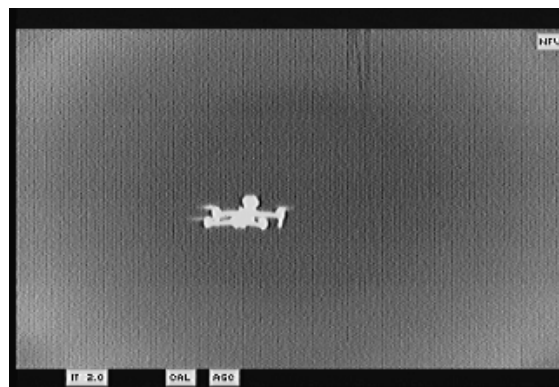
Figure 12 Footage of a DJI Mavic 2 Enterprise captured by a MATIS MWIR camera during the night
