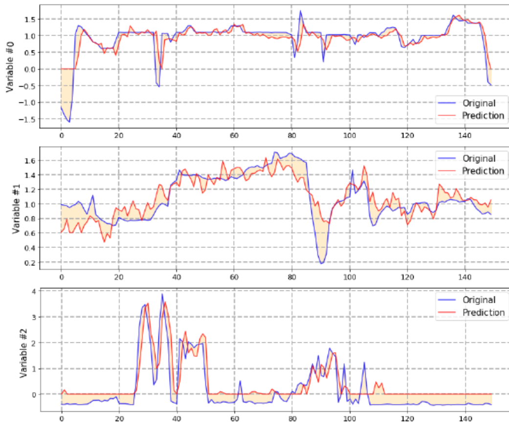
Figure 3-3. Long-Short Term Memory Networks (LSTM) prediction output (red) versus the real value to be predicted (blue) for three attributes of the diesel engine for propulsion. X-axis represents normalized data coming from the BAM ship; Y-axis contains an ordered index. Shaded area represents prediction error.
