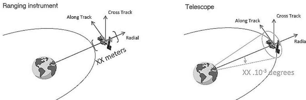
Figure 2: Definition of the precision in the estimation of the location of a satellite using a ranging instrument or a telescope [6].
