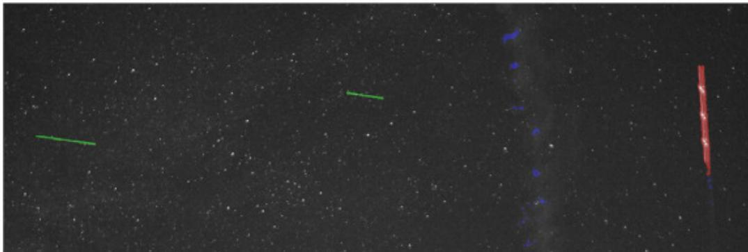
Figure 7: LEO objects detection. Sample result. Objects detection and automatic classification: two LEO objects (left) identified by the green colour, irrelevant objects identified by blue (right) and an airplane identified by red (right).
