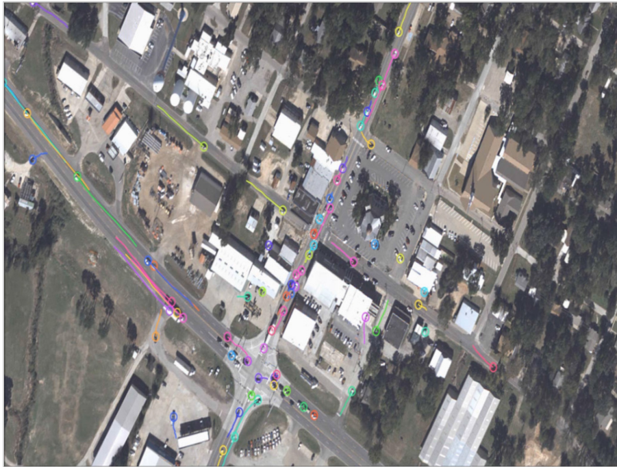
Figure 4: Example of vehicles being tracked and displayed in a ROI.
