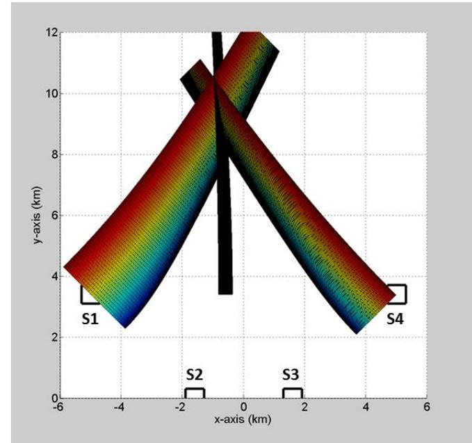
4 receivers in a “forward-looking” system configuration,
