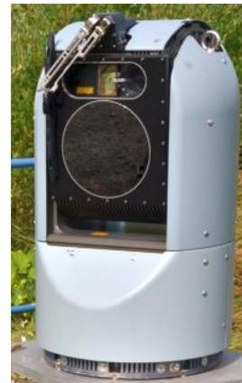
Figure 11: right: stabilized Multi Sensor Platform for Naval & Air Defence applications
