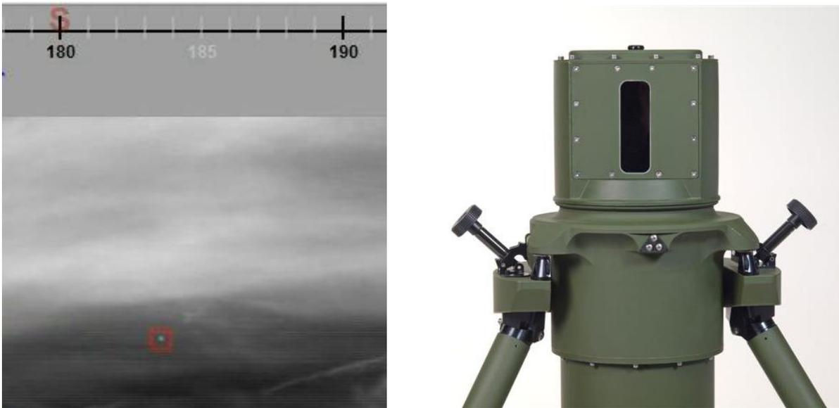
Figure 5: FIRST “hot spot” detection of an LSS-UAS (circled in red)
