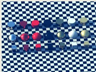
Example of different reflectivity settings available in DIRSIG, including spectral, diffuse, and custom BRDF modeling
