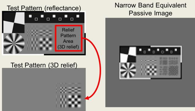
The virtual target (upper left) was used to simulate 2D and 3D active imaging systems (see sections to the right). The portion of the target outlined in red has a 3D relief pattern (shown bottom left).
