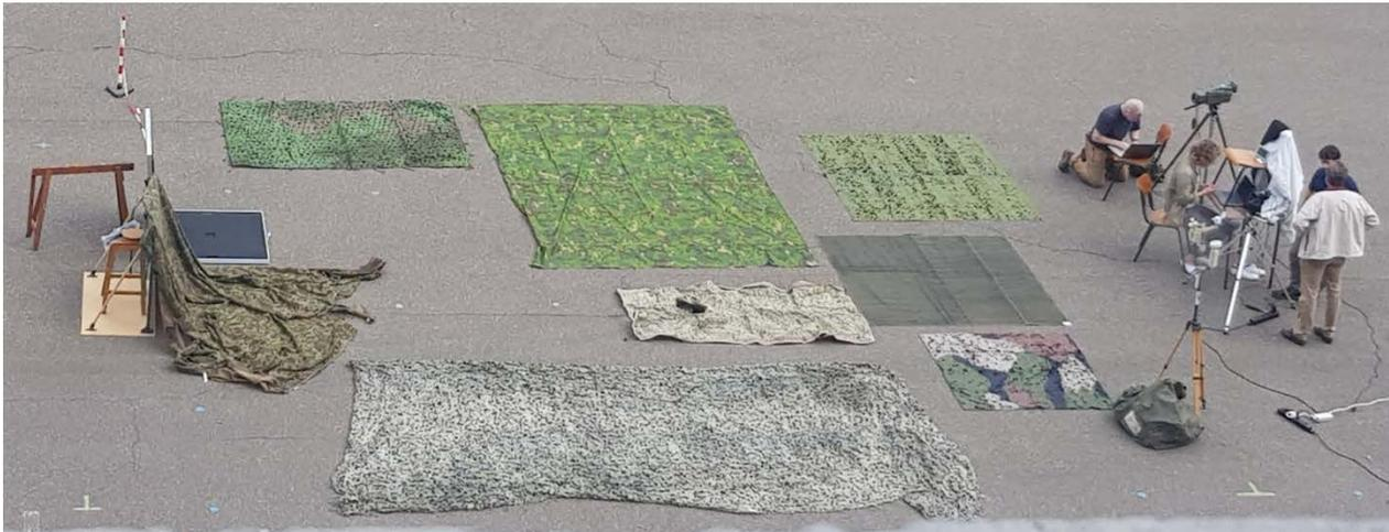
Figure 3-1: Outdoors nets measurements with calibrated reflectance panels.
