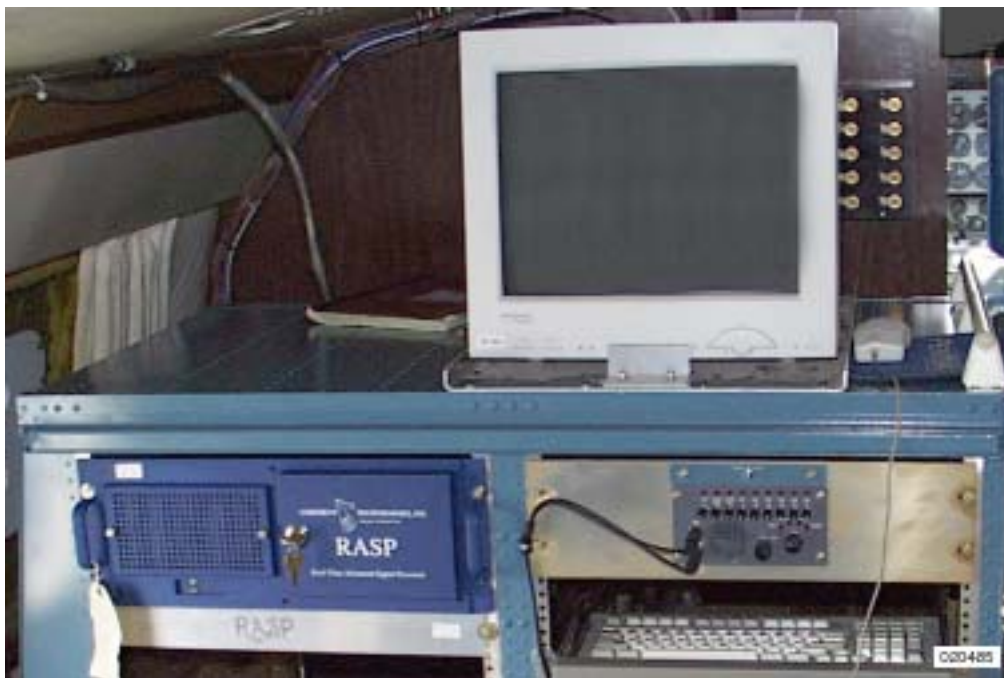
Figure 4-1: Flight-qualified real-time advanced signal processor (RASP) and display.
