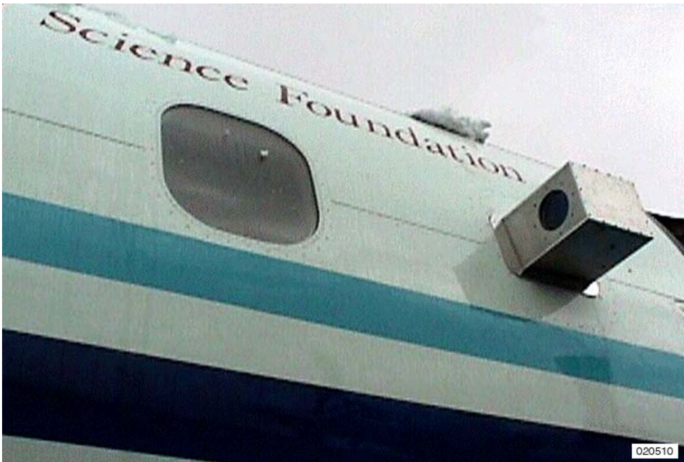
Figure 7-7: Folding mirror housing on the Electra testbed aircraft.
