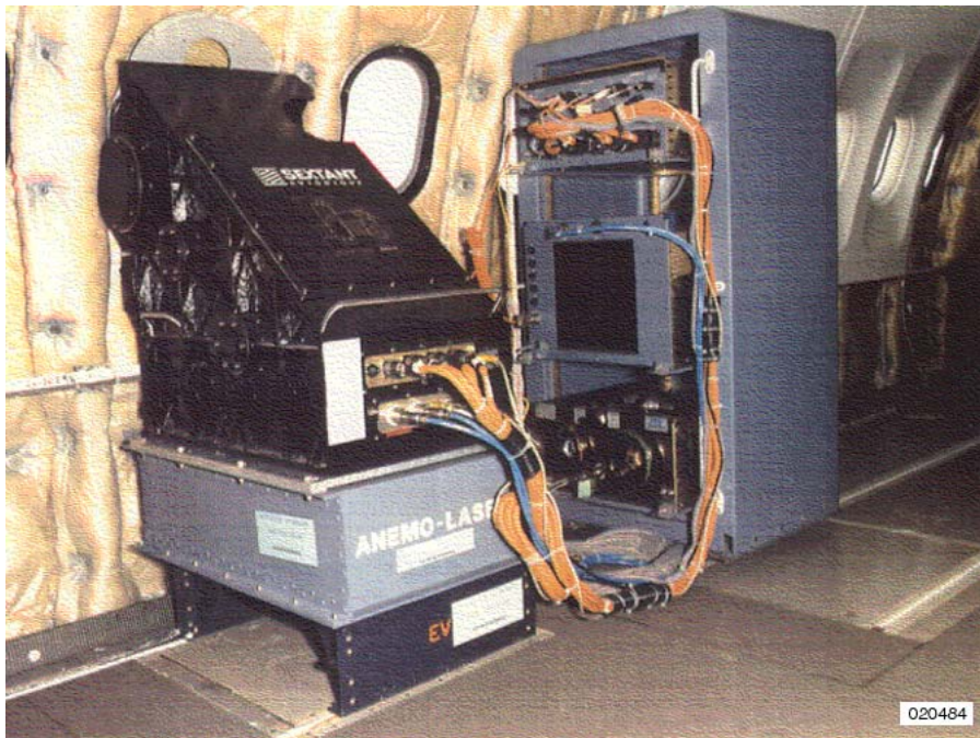
Figure 7-2: Installation of ALEV 3 system in the Airbus A340.
