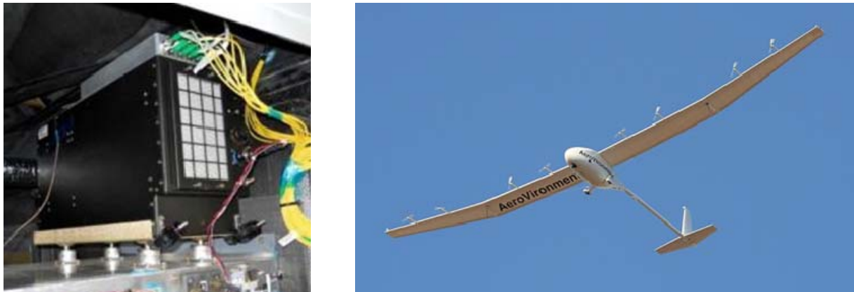
Figure 6-7: Flight Interrogation Unit and the Global Observer UAV.
