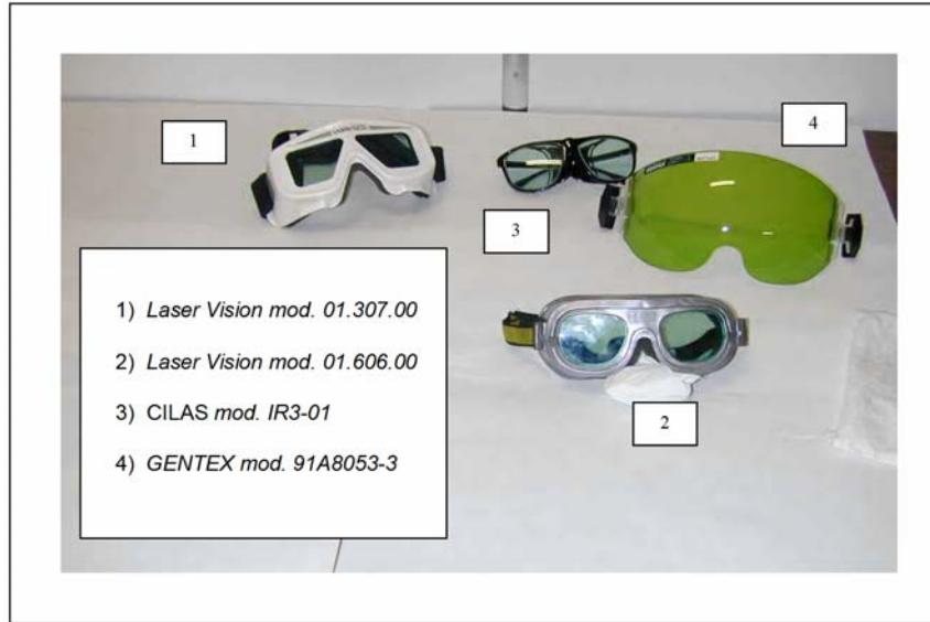
Figure 7-39: Tested Laser Protection Filters.
