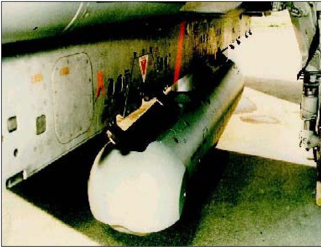
Figure 2-3: TORNADO-IDS CLDP Installation.
