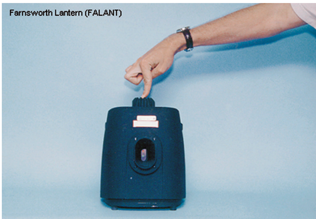
Figure A2.8: The Farnsworth Lantern is a screening tool for red-green colour defects. It is a rather liberal test, but has the advantage of not requiring special lighting conditions since the illuminator is contained in the apparatus.
