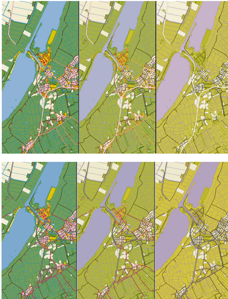
Figure 3.4: A map display, as seen by the normal trichomat (left), a deuteranomalous trichomat (middle) and a deuteranope (right). Upper row: original map, showing the gradual disappearance of the (orange) secondary roads with increasing deficiency (from anomalous to dichromatic). Bottom row: slightly adjusted map (orange replaced by dark red), showing the improved visibility of the road structure, both for dichromatic and anomalous colour vision.
