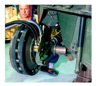
Figure 7.10: Roadwheel Integrated PEM Motor.
