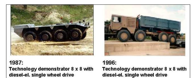
Figure 7.2: Electric Drive System in Wheeled Vehicles.
