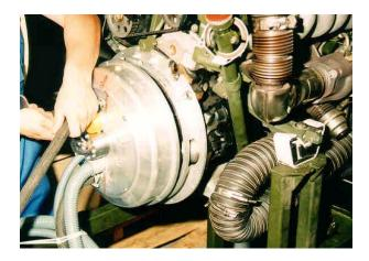
Figure 7.9: Diesel Engine Integrated PM Generator.
