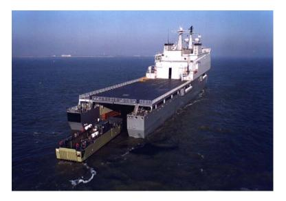
Figure 8.1: LPD HMS Rotterdam of the Royal Netherlands Navy with 15 MW Propulsion.
