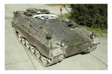
Figure 7.6: APC-Prototype MARDER with Diesel-Electric Propulsion.
