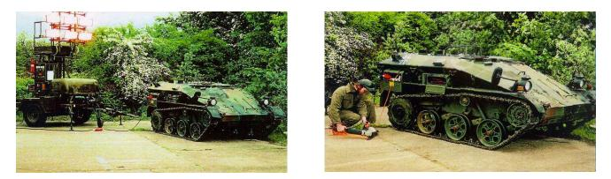
Figure 7.8: LLX-Prototype Wiesel with Diesel-Electric Propulsion and External Power Supply (DC/AC).
