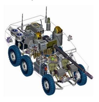
Figure 6.12: Virtual Prototype of Hybrid Electric System.
