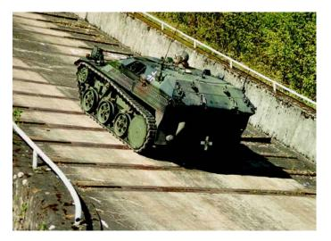
Figure 7.12: The Wiesel LLX in a 60% Slope.
