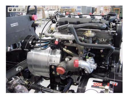
Figure 7.1: Hybrid HMMWV Engine/Generator.
