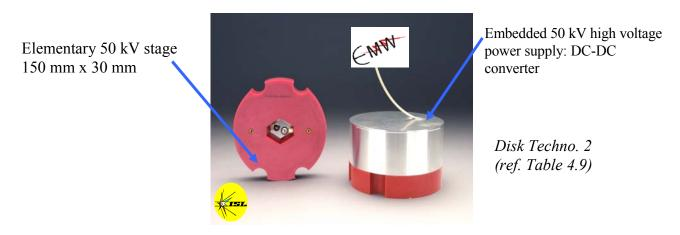
Figure 4.9: View of One Elementary EMW Marx Stage. Each stage includes the charging resistors and the two half-spark gap spheres.
