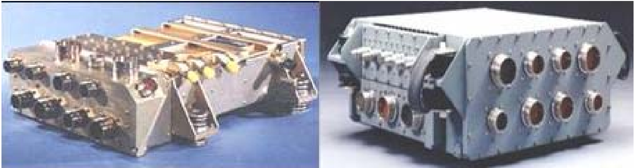
Figure 4.3: FADEC Examples from the F414 and CFM56 Engines. Note the highly ruggedized packaging, closely spaced I/O connectors, and heavy isolation mounts which all contribute to C&A weight.
