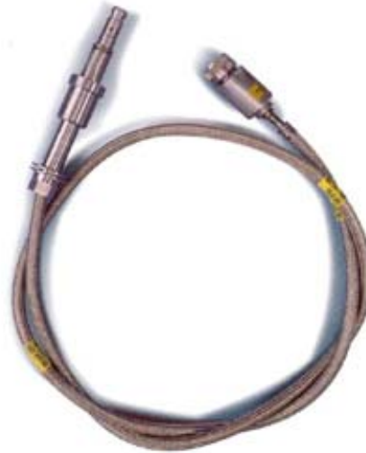
Figure 6.4: Radiation Pyrometer for EJ200 Engine for the Eurofighter Typhoon [6.6].
