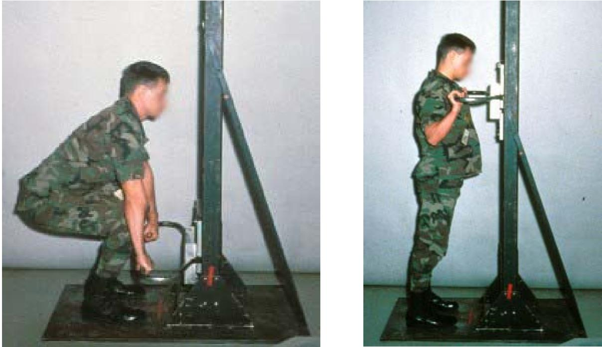
**Figure 5-4: Incremental Lift Machine (Starting and Ending Position).**
