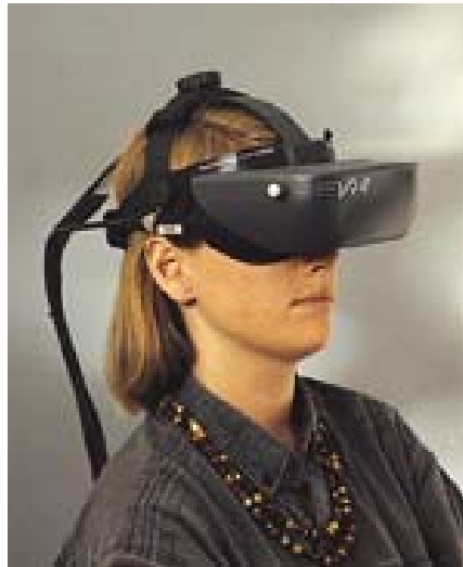
Figure 15: SMI iView – Head-Mounted Display with Integrated Eye Tracking Device. (Adopted from the Website of Sensomotoric Instruments GmbH, http://www.smi.de )
