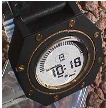
Figure 7: Sleep Watch Actigraph showing Fuel Gauge-Type Current Performance Capacity Readout.
